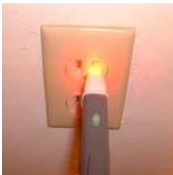
Non-Contact Voltage Sensing Pen Tester
