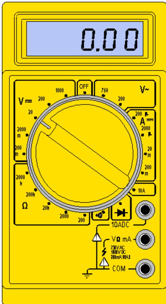
The central knob has lots of positions and you must choose which one is appropriate for the measurement you want to make. If the meter is switched to 20 V DC, for example, then 20 V is the maximum voltage which can be measured. This is sometimes called 20 V fsd (full scale deflection).
