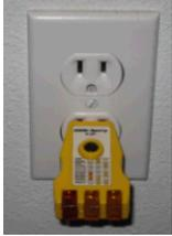
Electrical receptacle testers are used to check for proper wiring at electrical receptacles as well as to check the function of GFCI's.
