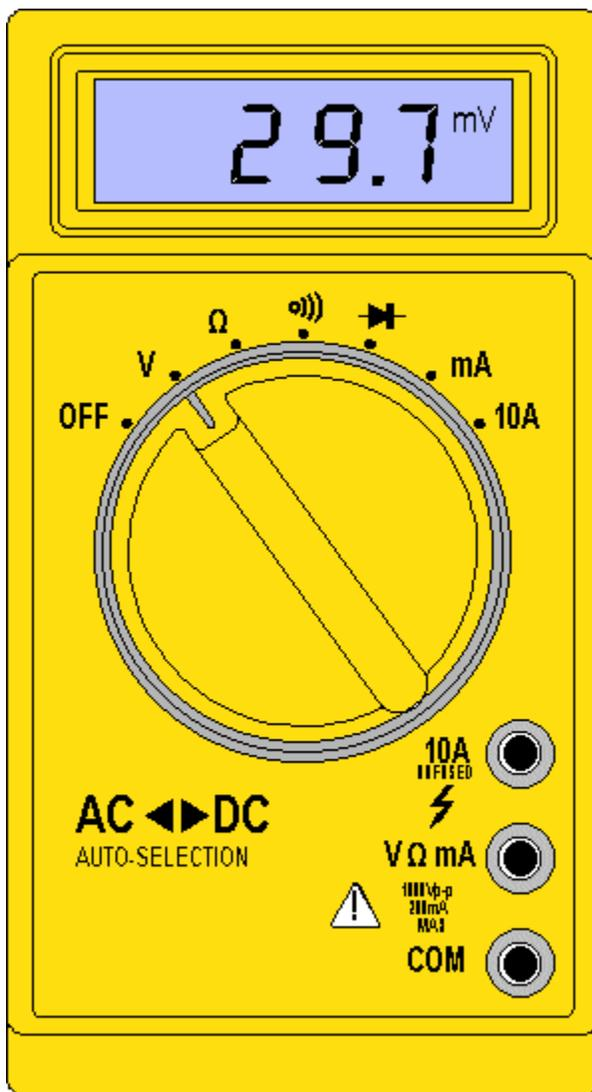
The central knob has fewer positions and all you need to do is to switch it to the quantity you want to measure. Once switched to V, the meter automatically adjusts its range to give a meaningful reading, and the display includes the unit of measurement, V or mV. This type of meter is more expensive, but obviously much easier to use.
